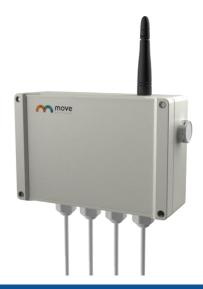
The Analog Node is designed to make geotechnical probes suited for LoRaWAN wireless communication, making it perfect for any geotechnical monitoring need. It is wireless, battery-powered, and plug-and-play.
