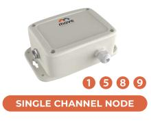
It makes geotechnical and environmental probes suited for wireless communication, sending alarms when a certain activation threshold is exceeded.
