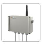
The Analog Communication Node is a wireless device that enables all connected sensors (originally wired) for wireless LoRaWAN communication. The Analog Node has a maximum of 4 channels supported and it is compatible with most of the analogue interfaces used for geotechnical sensors. The Analog Communication Node transmits accurate readings from all sensors connected via the LoRaWAN wireless communication protocol to the Gateway.
